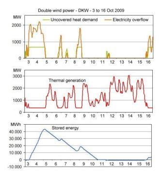
700 MW of the remaining variation can be utilized for uncovered heat demand while up to 1,500 MW are assumed to be absorbed by hot water storages.
