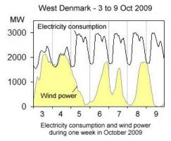
Finally we must aim at an efficient utilization of the additional wind energy. Twice the wind power on the chart will during certain periods create a surplus of electricity which should be utilized the best possible way to the benefit of environment.
