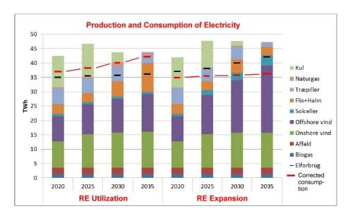
In RE Expansion more than 10 TWh must be exported every year from 2025. In RE Utilization it has been possible to utilize an increasing amount of electricity within Denmark and to reduce the overflow in 2035 to an insignificant level. Besides the share of CHP in the district heating systems is much higher. It is strange that the 5 points conclusion does not recommend an RE utilization policy.
