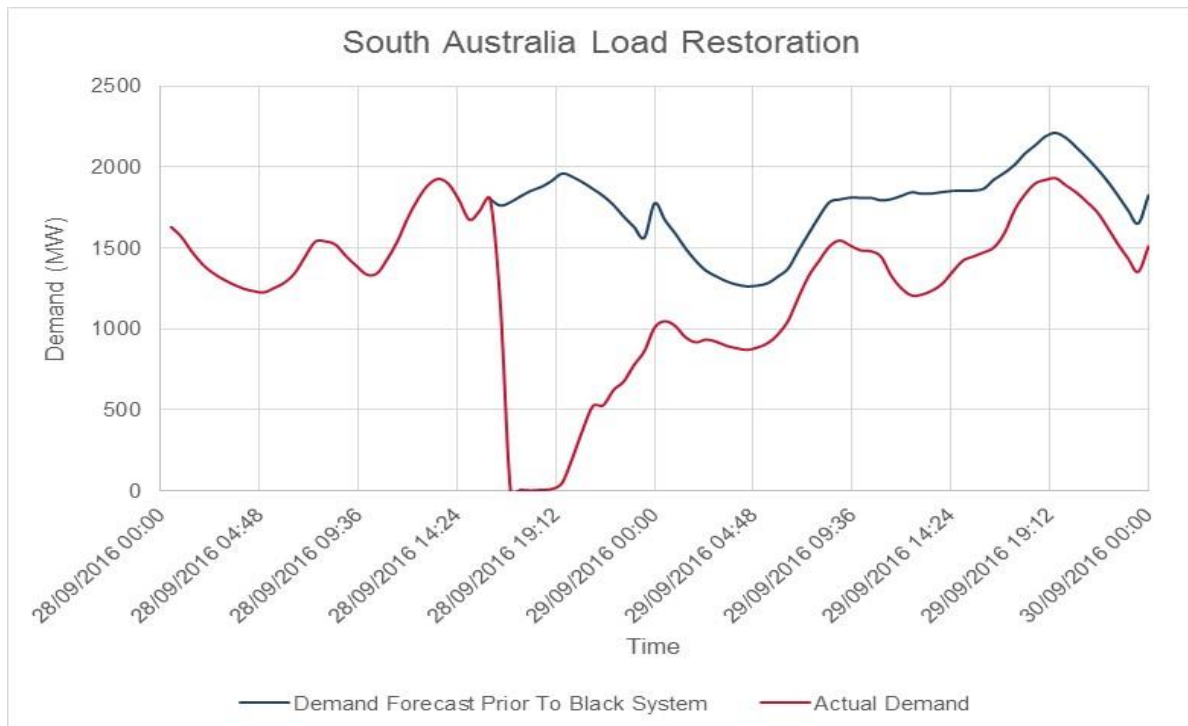
Figure 23 Comparison of forecast and actual load
