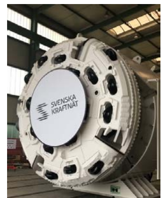
Fig. 5 - SKN drill for tunnel
