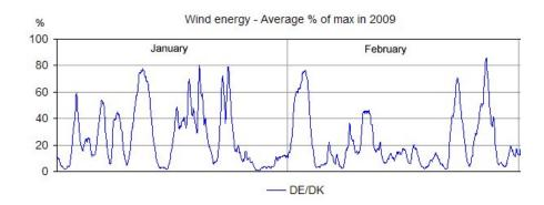
The chart shows the volatile and random nature, even for the average wind power output for Germany and Denmark. The duration of typical wind power waves can be between 2 and 4 days. The peaks are slightly lower than for each country, but there are still periods with very low generation and several days with less than 20 % energy output.
