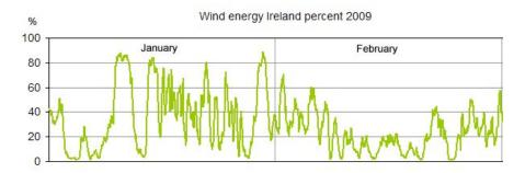
There seem to be some oscillations with higher frequency than what has been seen in Denmark and Germany. The variations could be connected with the number of wind farms and the distances between locations in Ireland rather than with special wind properties.
