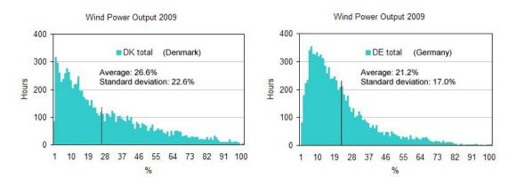
The average in Germany reflects the lower average wind intensity at the wind power sites. The standard deviation depends on the size of the country. It is obvious from the chart that Germany has a lower number of hours with very low and very high total output.
